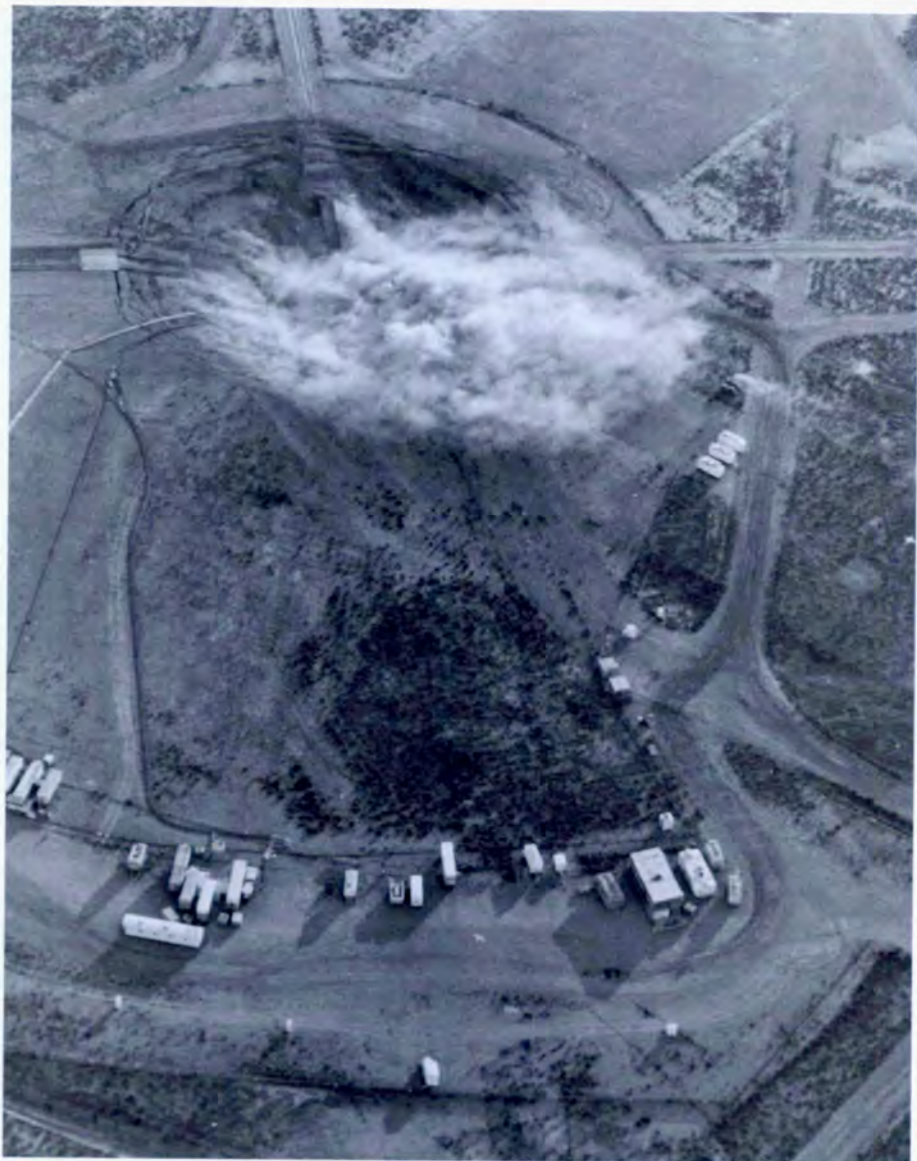
Aerial view of the formation of a postshot subsidence crater at the moment of collapse. This collapse may occur from a few minutes to many hours after a shot is fired. Note the dust caused by falling earth.
